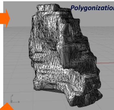
Convert into polygon mesh using 3D-DOCTOR™
